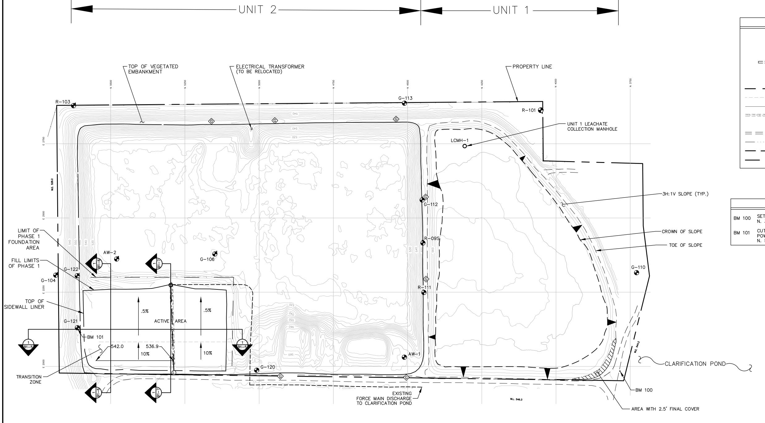
LEGEND BENCHMARK (SEE DESCRIPTION THIS SHEET) GROUNDWATER MONITORING WELL (EXISTING) PIEZOMETER (LONG TERM) CULVERT LEACHATE COLLECTION MANHOLE LEACHATE CLEANOUT RISER LEACHATE COLLECTION LINE TRENCH INVERT GRADE BREAK POINT FENCE FOUNDATION UNDERDRAIN LATERAL FOUNDATION UNDERDRAIN COLLECTION RISER = = = ROADWAYS STREAM, DITCH OR WATERWAY PROPERTY BOUNDARY UNIT 2 WASTE BOUNDARY
